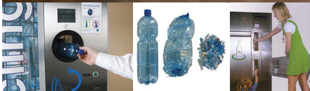
Top: reVend & Spend machine. Above from L-R: Bottles are inserted into the machine and reduced in size. The machines can be used for front-of-house recycling in supermarkets.
